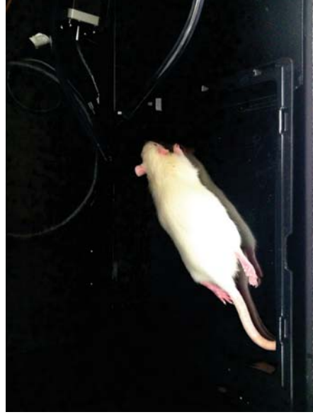
Corner nose cone allows for diagonal positioning to maximize imaging field of view (FOV). 200 g rat shown.
