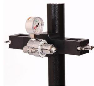
Remove the 2 stainless steel screws from the manifold and use them to attach the manifold assembly onto the anesthesia machine pole. Tighten using the Allen wrench provided with the manifold. Note that the manifold should be positioned on the back side of the anesthesia machine. See photo showing location of manifold in relation to machine head.
