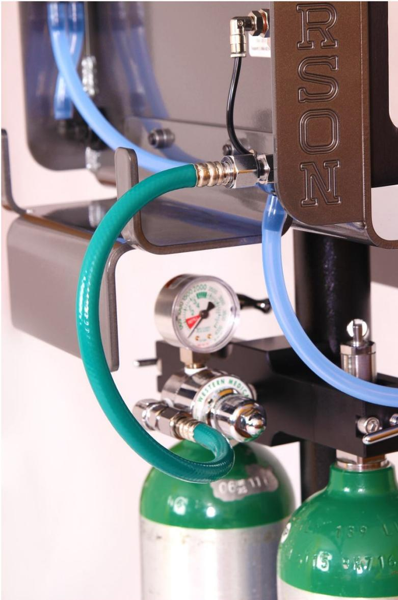
Connect the short green O<sub>2</sub> hose between the DISS fitting on the regulator outlet and the DISS fitting on the inlet of the anesthesia machine. Hand tighten both ends of the hose and then snug tight with a wrench.
