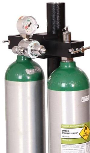
Insert E sized oxygen cylinders into the ends of the manifold, noting the location and orientation of the indexing pins, and lock into place with the chrome T handles.
