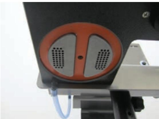
Remove absorber canister and wipe gasket clean with isopropyl alcohol. Examine holes for any blockage from CO<sub>2</sub> absorbent.
