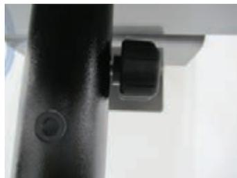
Remove the anesthesia machine head from the packaging and place the mounting "spud" into the top of the pole.
