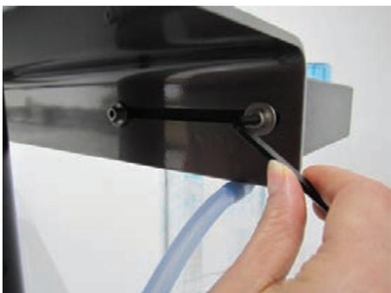
Remove both 1/4-20 socket head cap screws securing absorber block to the frame.
