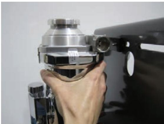
Lift vaporizer and thread screws into the vaporizer manifold. Hand tighten only at this point.
