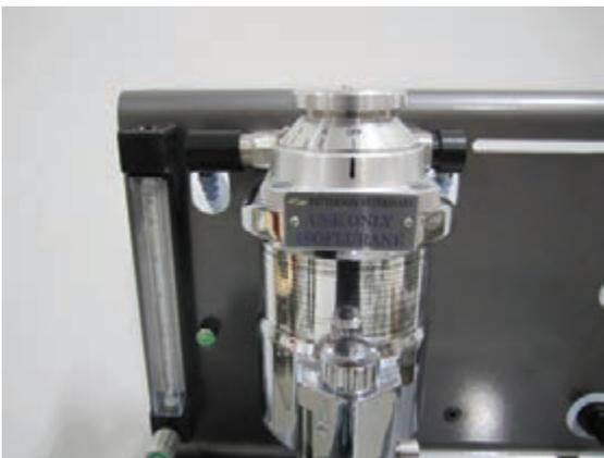
Vaporizer should be positioned as shown with the tubing centered in the slots.
