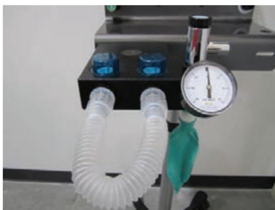
3. Pressurize the absorber system until the manometer reads 30 to 40 cmH<sub>2</sub>O.
