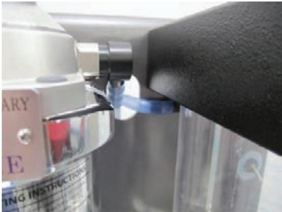
Mount absorber assembly to the slot on the right side of the vaporizer mounting area using the same 1/4–20 socket head cap screws. Route silicone tubing through the hole next to the outlet side of the vaporizer and connect the open end to the T-piece where it was originally connected.
