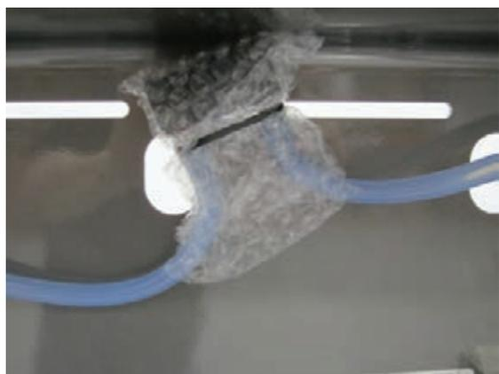
Cut cable tie and remove bubble bag to expose endcaps.
