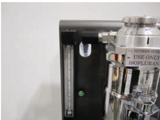
Install female endcap onto the inlet side of vaporizer manifold. Move vaporizer so that the tubing is centered with the slot as shown.
