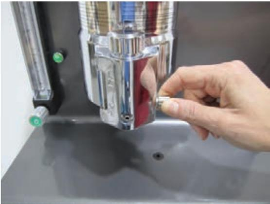
Tighten drain stem as shown.
