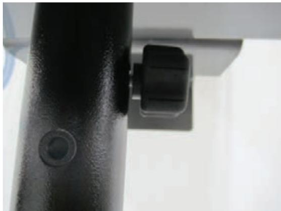
Remove pole knob and lift the head of the anesthesia machine off of pole and place it on a table or countertop.
