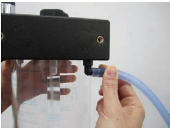
Turn elbow connector 90° clockwise (as viewed from bottom of absorber block). Hose barb will point away from absorber canister.
