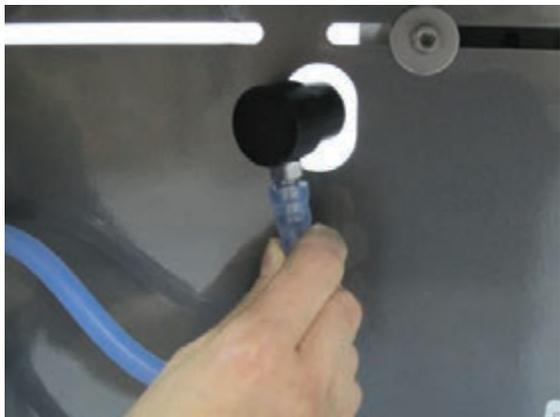
Push male endcap through other slot and attach to outlet side of vaporizer.
