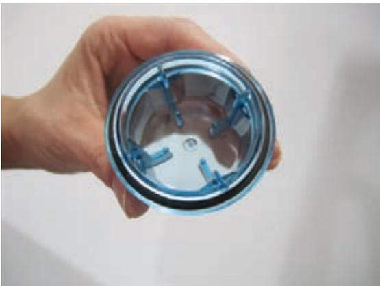
Clean dome cap O-rings and all internal/external features with a mild soapy water solution and dry before reinstalling.
