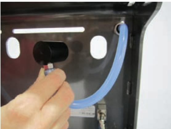
Push female endcap through large slot next to the flowmeter. Female endcap should now be positioned on the other side of frame as shown in the next picture.
